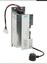
The QE20-FP2001 PSU Module can be fitted as an additional power supply when expanding a QE20 system, or as a replacement for an existing PSU module. A QE20-FP2027 fused power distribution board can be fitted to the PSU to provide 4 independently fused outputs for field wiring or other uses. The QE20-FP2001 PSU Module provides a regulated 26VDC to power up to 480W of amplifier load. Up to 4 PSU may be connected to the same battery in the same cabinet.
